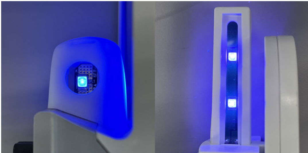
FIGURE #3: LED appearance of expensive insect trap sample (left) and affordable insect trap sample (right). The expensive insect trap LED appears to be a deeper shade of blue, potentially indicating a peak wavelength deeper in the UV region.
