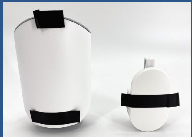
FIGURE #1 Insect trap samples used in the experiment: a higher-cost model (left) and a more affordable model (right). Tape was added to cover branding for the figure but was not used during measurements to avoid affecting LED readings.
