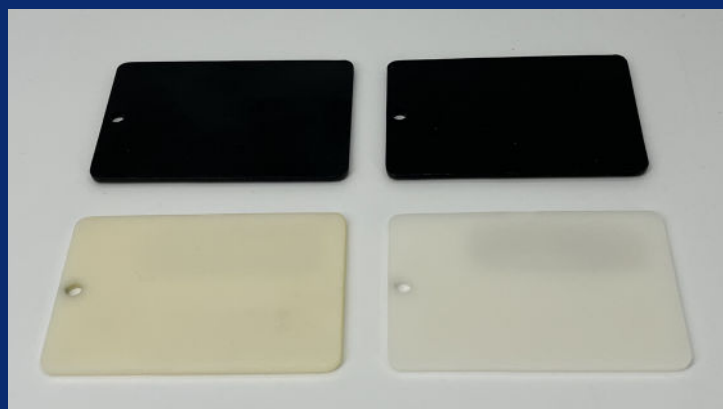
FIGURE #1 Plastic samples used for this experiment, including black ABS (top-left), black Delrin (top-right), white ABS (bottom-left), and white Delrin (bottom-right).
