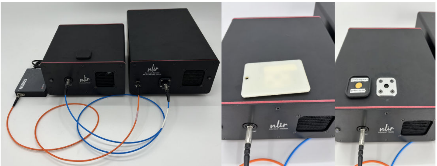
FIGURE #2 Experimental setup for plastic measurements. The spectrometer was connected to the NLIR SPEKTRUM via fiber optic cable, while the SPEKTRUM connected to the TOUCH measurement device. Samples were measured by placing them directly on the TOUCH surface, which includes an integrated gold reference tile for convenient referencing.
