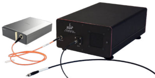
NLIR's SPEKTRUM Wavelength Converter coupled to Avantes AvaSpec-VARIUS™ Spectrometer.
