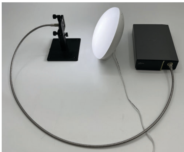
FIGURE #2 Experimental setup for lamp measurements.
