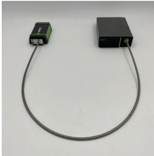
FIGURE #3 Setup for irradiance calibration. The spectrometer was attached to the fiber optic cable, which was then attached to the calibration source. The calibration source had a cosine corrector in-line, which was the one used for all following radiometric measurements.
