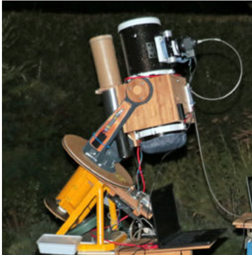
Figure 3: Ground-based setup: a 150 mm Newtonian telescope coupled via optical fiber to an Avantes NEXOS™ spectrometer. The system was mounted on a custom-built equatorial fork mount and aligned using a guiding camera for accurate tracking.
