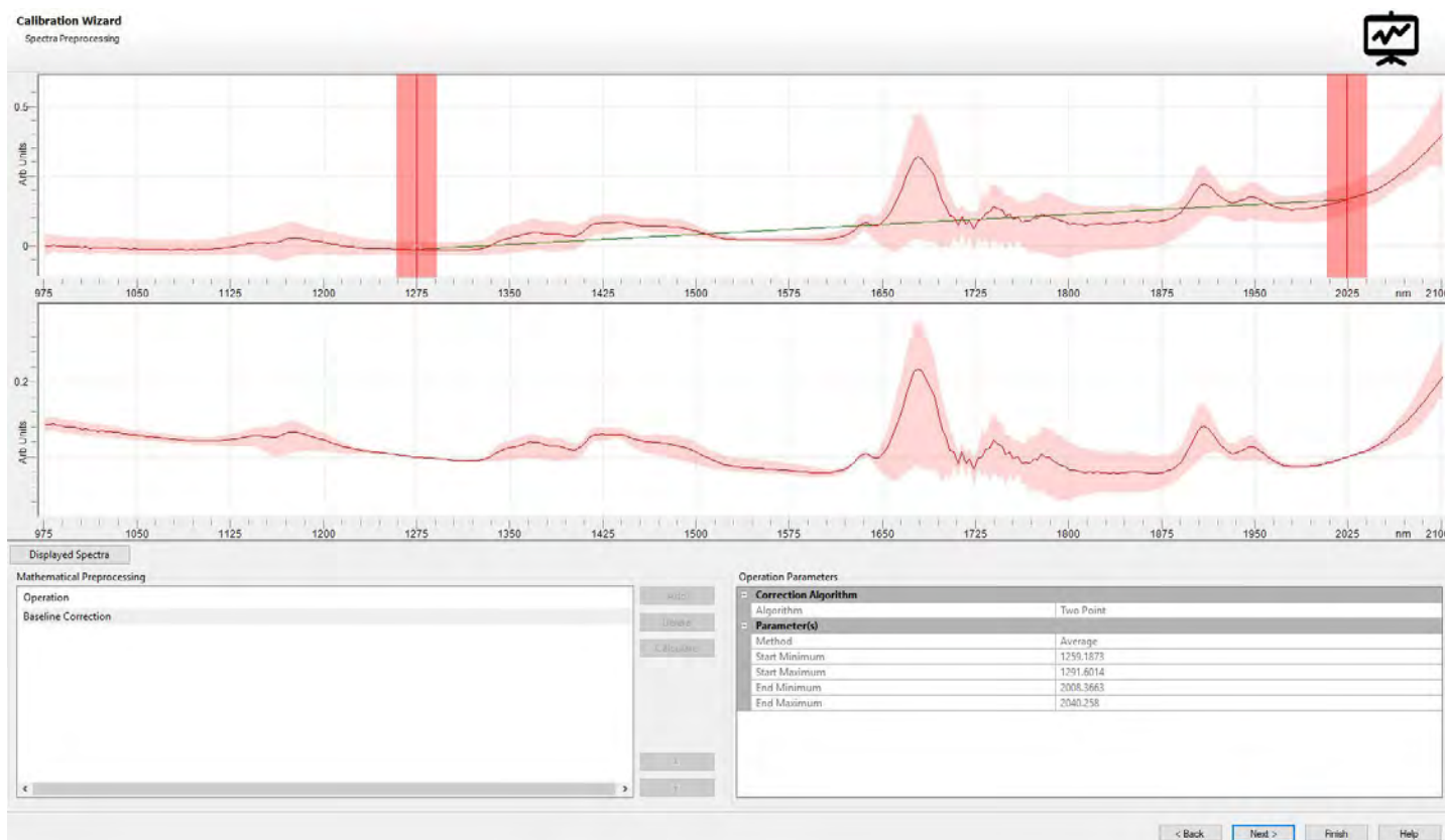
Figure 3: The spectra processing screen of Panorama, where the mathematical operations can be manipulated.
