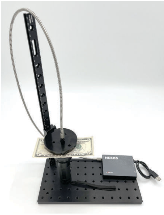
FIGURE #2 Experimental setup for fluorescence measurements: A spectrometer connected via fiber optic to a collimating lens and filter holder was aimed at the bill's fluorescent stripe. The bill was placed over a UV flashlight to enhance fluorescence.
