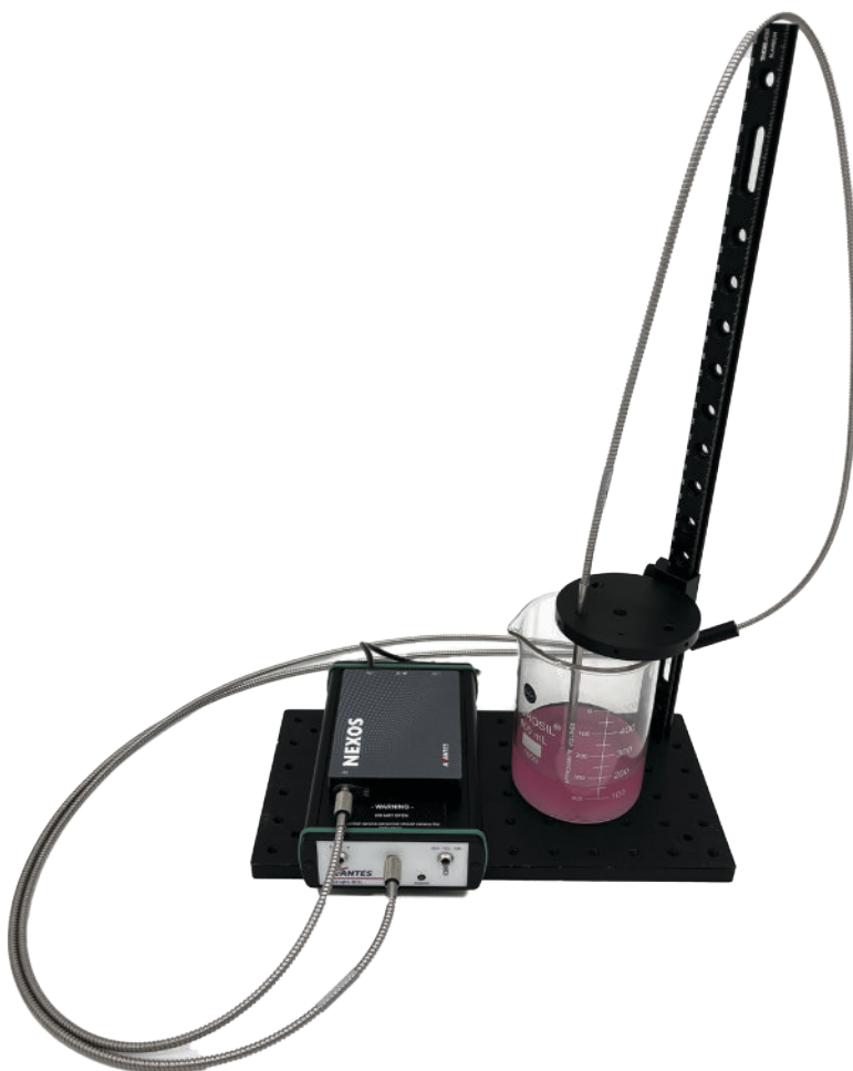
FIGURE #2 Experimental setup for the absorbance measurements. The spectrometer and light source are attached to the dip probe. The dip probe is mounted in the Transmission-Reflection (TR) Stage and immersed in the vitamin solution (vitamin B12 solution shown here) to perform a measurement.
