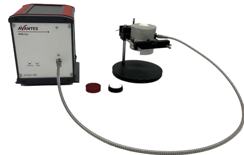
FIGURE #2: setup for flour measurements: samples were placed on glass slides over the integrating sphere port, connected to the NIR spectrometer via a fiber optic cable. A WS-2 reference tile served as the reference, and a BS-2 tile (not pictured) was used for the dark measurement
