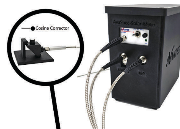
FIGURE #2 Experimental setup for solar simulator measurement: The spectrometers, AvaTrigger, and interface cable were housed in a custom enclosure. A custom fiber optic cable connected the spectrometers and AvaTrigger to the 90-degree cosine corrector and collimating lens, both mounted in a 3D-printed holder.
