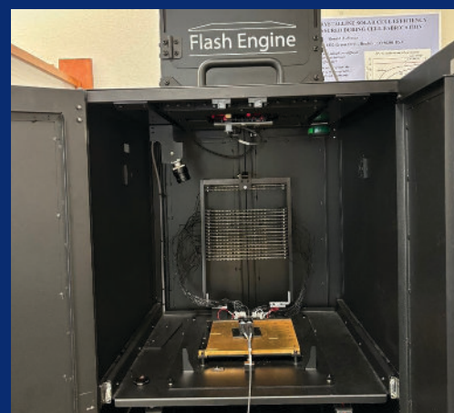
FIGURE #1 Measurement setup showing the placement of the measurement end inside the solar simulator.
