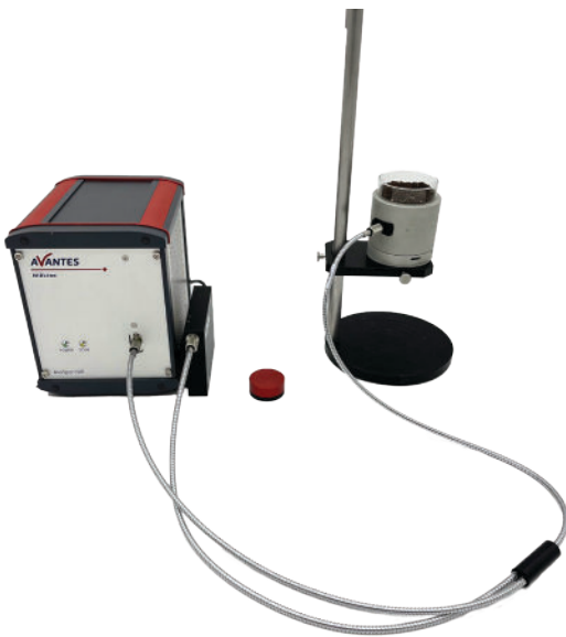
FIGURE #2 Experimental setup: Soil samples are placed in small petri dishes and measured within an integrating sphere with a built-in halogen light source.
