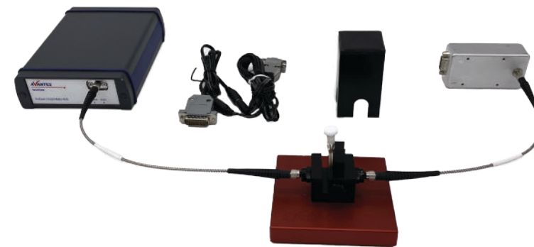
FIGURE #2 Spectroscopy Setup. The caffeine sample is placed inside a 1 mm path length cuvette, which is measured in-line using our cuvette holder and cuvette cover. The light source is controlled by the spectrometer via the interface cable.
