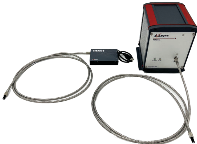
FIGURE #1 Experimental setup for snow sample measurements. Each spectrometer was irradiance calibrated with the attached fiber and cosine corrector. During the measurements, the fiber was pointed at the snow samples at an angle to measurement incident reflectance.
