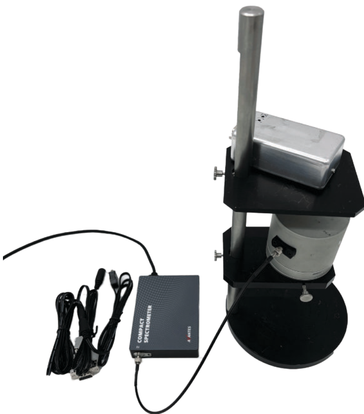
FIGURE #2 Experimental setup for clothing sample measurements. The clothing sample is placed directly on top of the integrating sphere sample port as the sample is exposed to UV light. The light source is controlled by the spectrometer via the interface cable.
