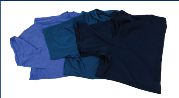
FIGURE #1: Clothing samples used for this experiment (from left to right: 50% cotton/50% polyester shirt, 100% polyester shirt, 100% polyester shirt with UV protective coating).
