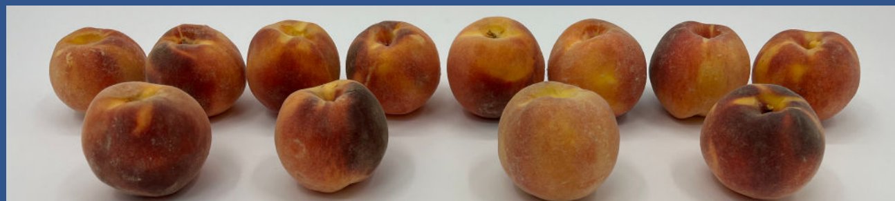
FIGURE 1 Peach samples used for this experiment. The eight peaches in the back row were those used to create the correlation between the measured spectra and sugar content, and the four peaches in the front row were those tested to determine the accuracy of our algorithm.
