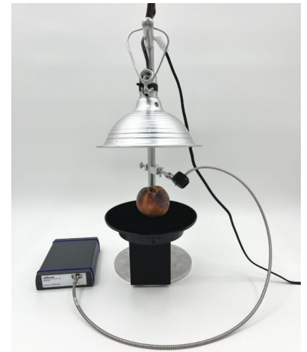
FIGURE 2 Experimental setup. One end of the fiber optic cable is connected to the spectrometer while the other is clamped and pointed at the peach sample. The peach samples are illuminated by the overhead lamp and are rotated via the turntable to take multiple measurements per sample.
