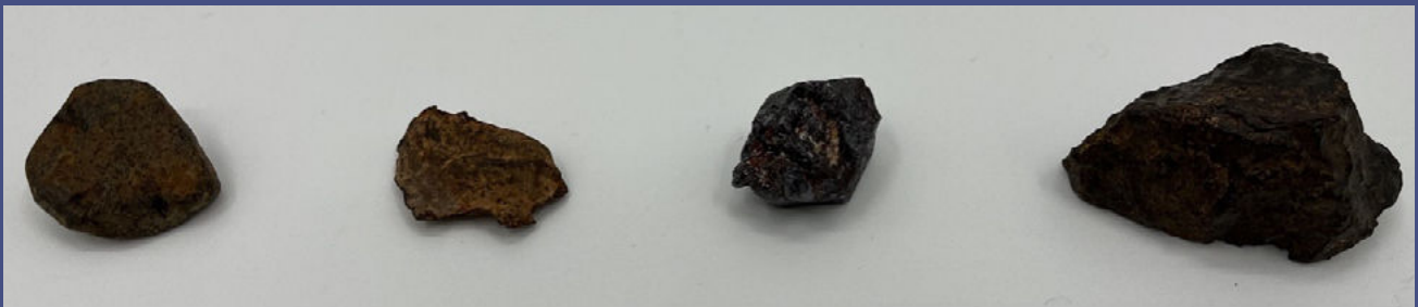
FIGURE 1 Rock and meteorite samples used for this experiment (from left to right: H5 ordinary chondrite, iron ataxite, iron oxide, and titanium dioxide) and Summer Gray).
