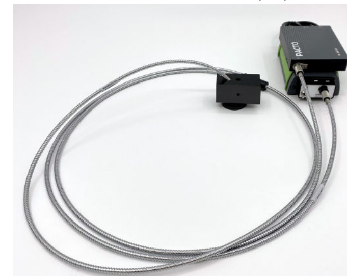
FIGURE #2 Experimental setup for tile measurement. The probe is mounted into the probe holder, which is then placed on top of the Oreo sample or reference tile.
