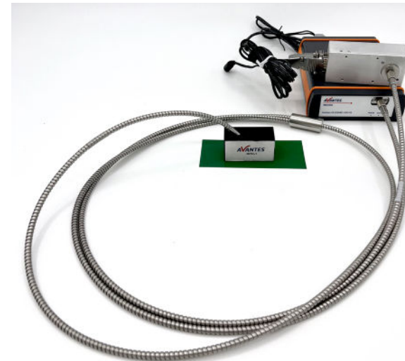
FIGURE 2 Experimental setup for paint measurement. Probe is mounted into the probe holder, which is then placed on top of the paint sample.
