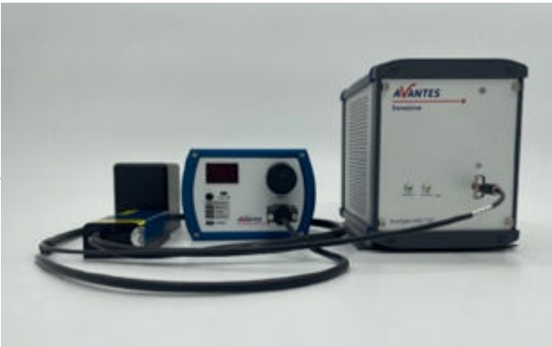
FIGURE 4: Set up of system with Raman 785 laser, AvaSpec-HSC, and sample holder
