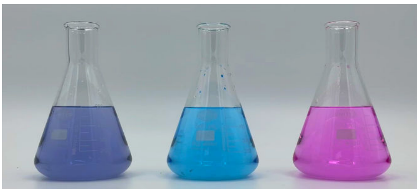
FIGURE 2: Initial colors of the pH indicators in basic solution
