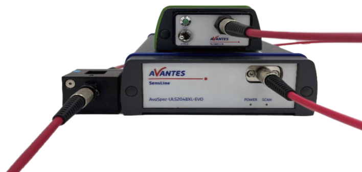
FIGURE 1 System Setup including Avaspec-ULS2048XL-EVO
