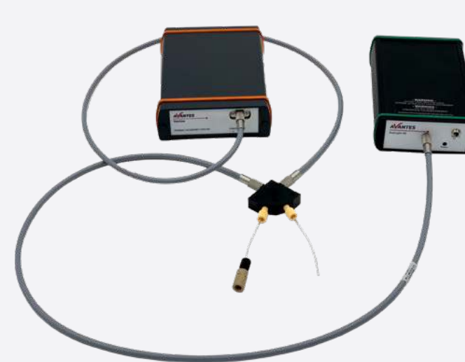
Figure 1: Microfluidic fluorescence set up with AvaSpec ULS2048CL-EVO
