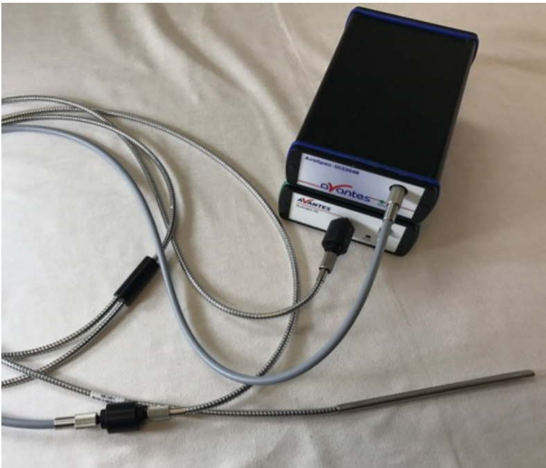
Fig. 4: Typical set-up fluorescence probe configuration
