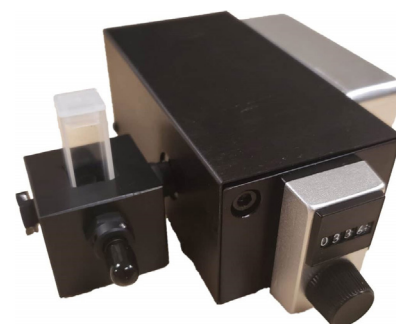
Figure 4: AvaFluorimeter accessory with built-in Xenon
