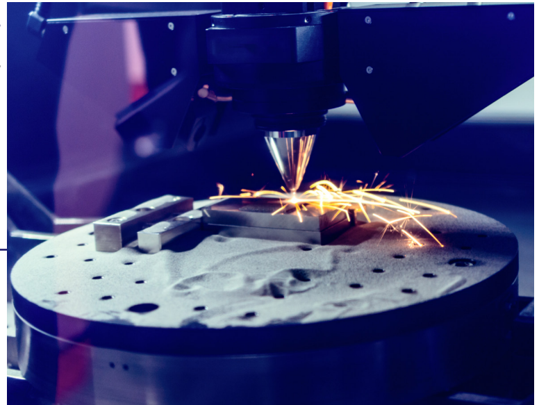
3D metal printer produces a steel part
